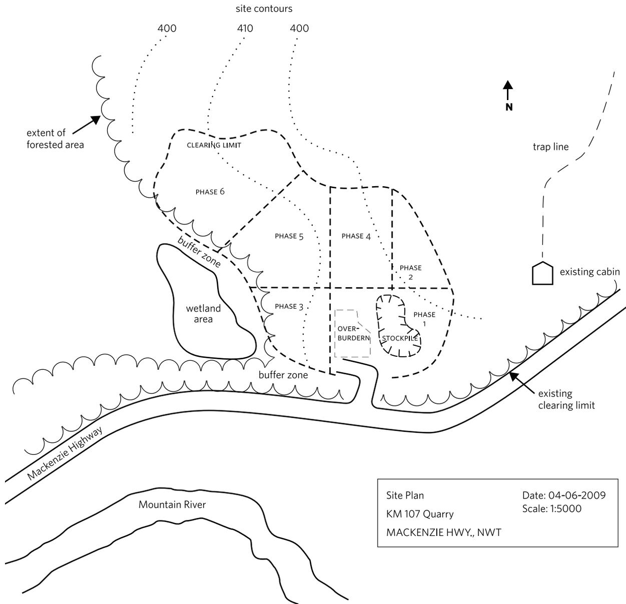
figure 14. Site design diagram to be submitted with a pit/quarry development plan. (Redrawn from Robertson and Brandt, 1997, p. 64.)
