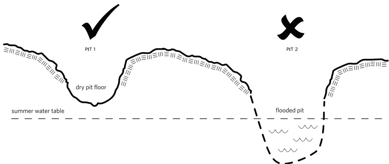
figure 13. Ensure pit excavation is well above the summer water table. (Redrawn from Robertson and Brandt, 1997, p. 31.)
