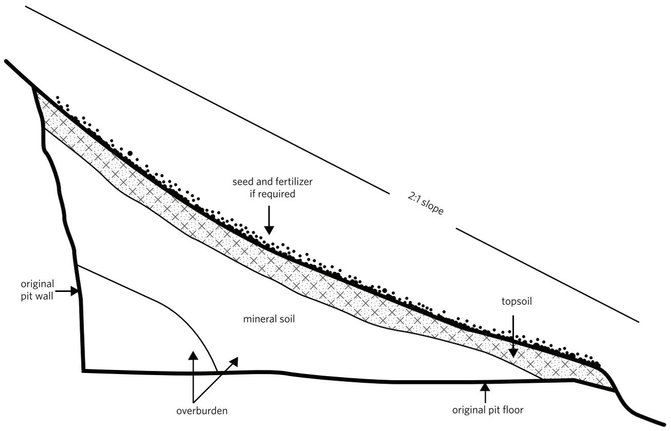
figure 26. Proper placement of overburden, mineral soil and topsoil for reclamation. (Redrawn from Robertson and Brandt, 1997, p. 42.)
