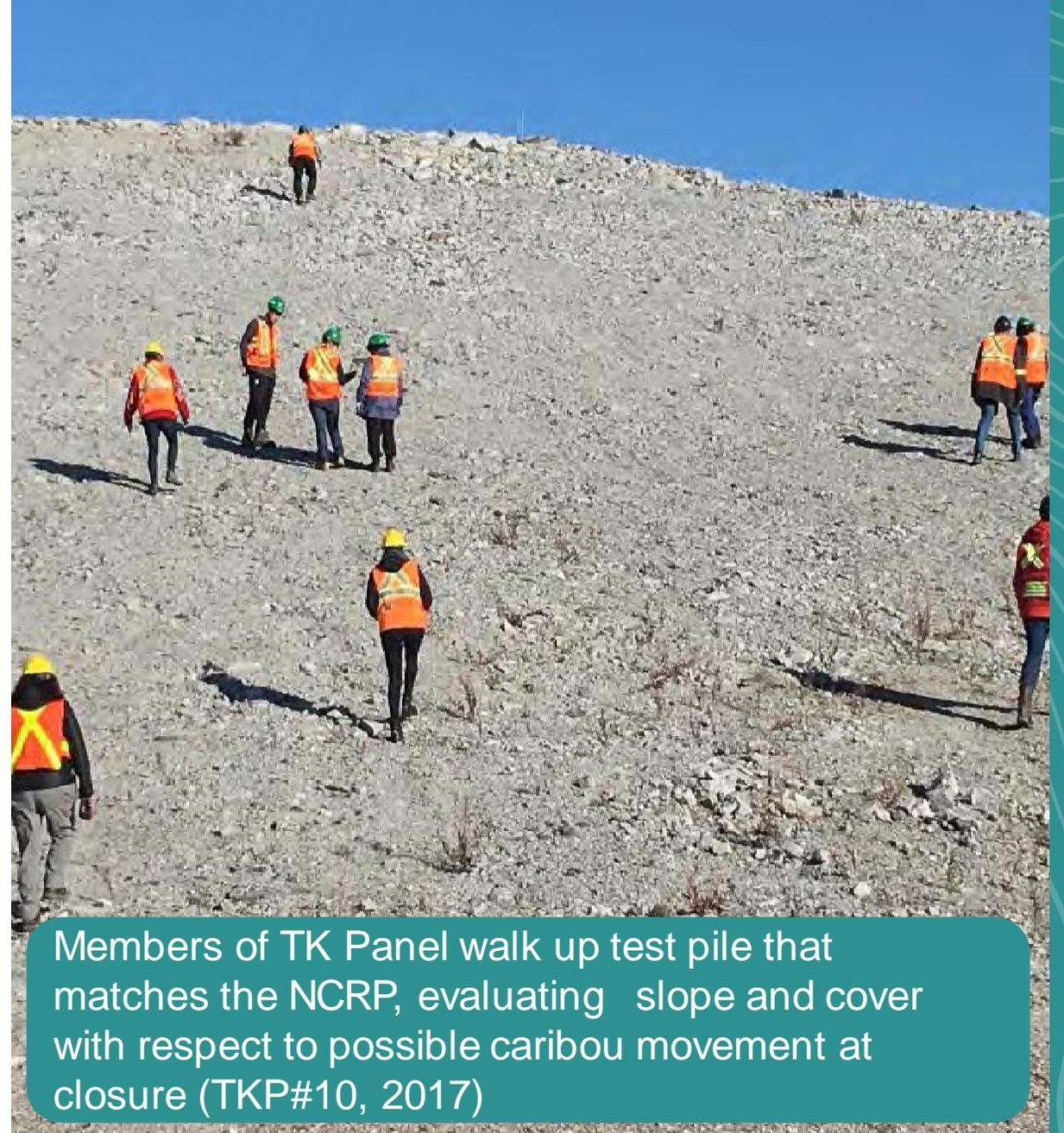
Members of TK Panel walk up test pile that matches the NCRP, evaluating slope and cover with respect to possible caribou movement at closure (TKP#10, 2017)
